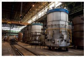
As the name suggests "Hydrogen Annealing" is notting but the annealing process which is carried out in ambient hydrogen atmosphere at elevated temperatures. Annealing is a heat treatment that is carried out to relieve internal stresses such as hot/cold shuts etc.All that were induced during fabrication process. (mostly during casting). This process involves three distinct microstructural changes in the material observed during controlled heating.
